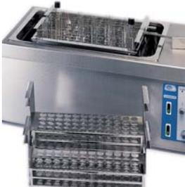
**Racks:** made of AISI 304 stainless steel.
