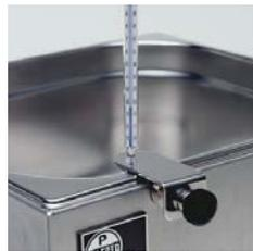
**Thermometer support with locking screw (up to 40 mm).**
