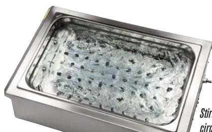
*Stirring detail by internal circulation pump.*
