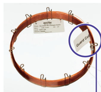
Tag indicates guard column end.
