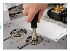
Simply slip the weldment removal tool over the weldment, then twist and remove the weldment. For speed and efficiency, the weldment stays secured in the weldment removal tool until you reattach it.
