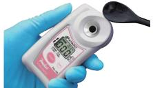
The PAL-10S is a digital hand-held compact refractometer that measures Urine Specific Gravity. To operate, simply place a drop of urine on the prism surface and press the START key. The Urine Specific Gravity value will be displayed on the LCD.
