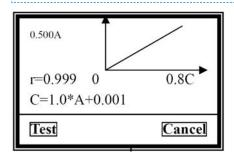
Graphic display visualized detail of a regression line for concentration calculation. (VR-2000)
