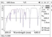
Graphic display visualized detail of holmium crystal scanning, from a UV3100 spectrophotometer.
