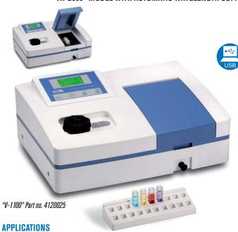
They are widely used in colleges and enterprises for general quantitatives analysis and experiments based in absorbance measurements.
