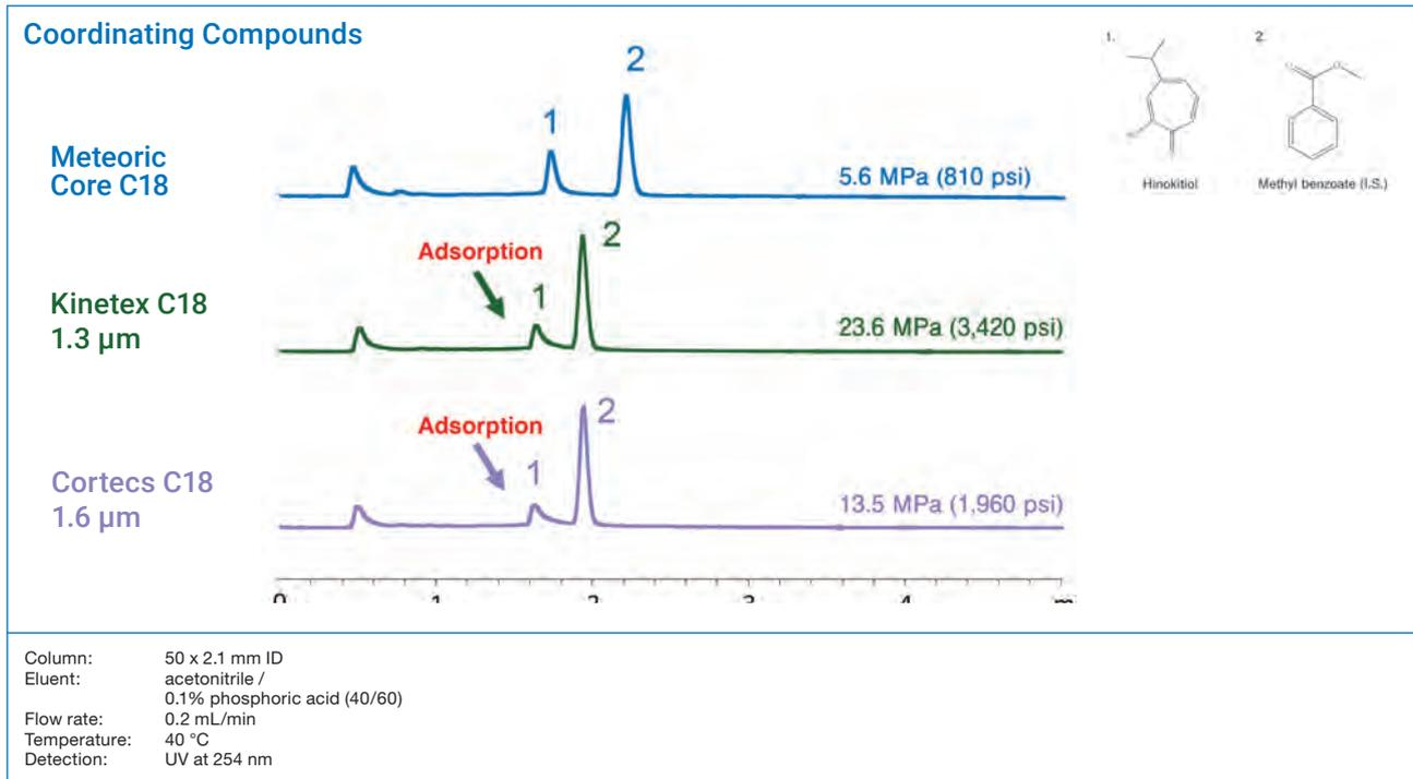
Meteoric Core C18 is able to provide excellent peak shapes for coordinating compounds which are often adsorbed by a column, as a result of a strong interaction with impurities such as trace amounts of metal ions. Meteoric Core is suitable for the quantitative analysis of coordinating compounds.
