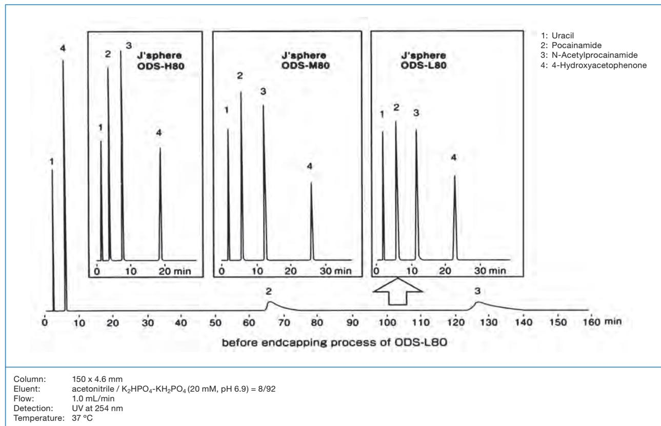
Three types of ODS are processed by endcapping technology to minimize the effect of residual silanol as much as possible.
