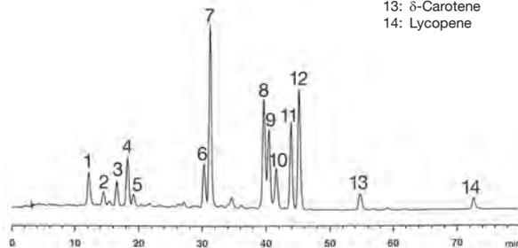
Column: YMC Carotenoid (5  $\mu$ m) 250 x 4.6 mm ID
