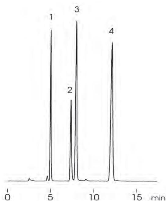
Column: YMC-Pack SIL (5  $\mu\text{m}$ , 12 nm) 250 x 4.6 mm ID
