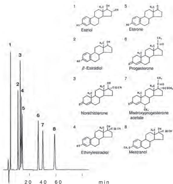
Column: YMC-Pack C<sub>8</sub> (Octyl) (5 μm, 12 nm) 250 x 4.6 mm ID
