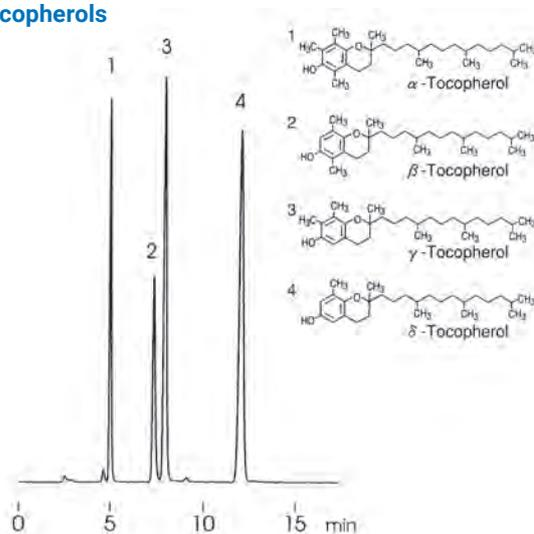
Column: YMC-Pack SIL (5 µm, 12 nm) 150 x 4.6 mm ID
