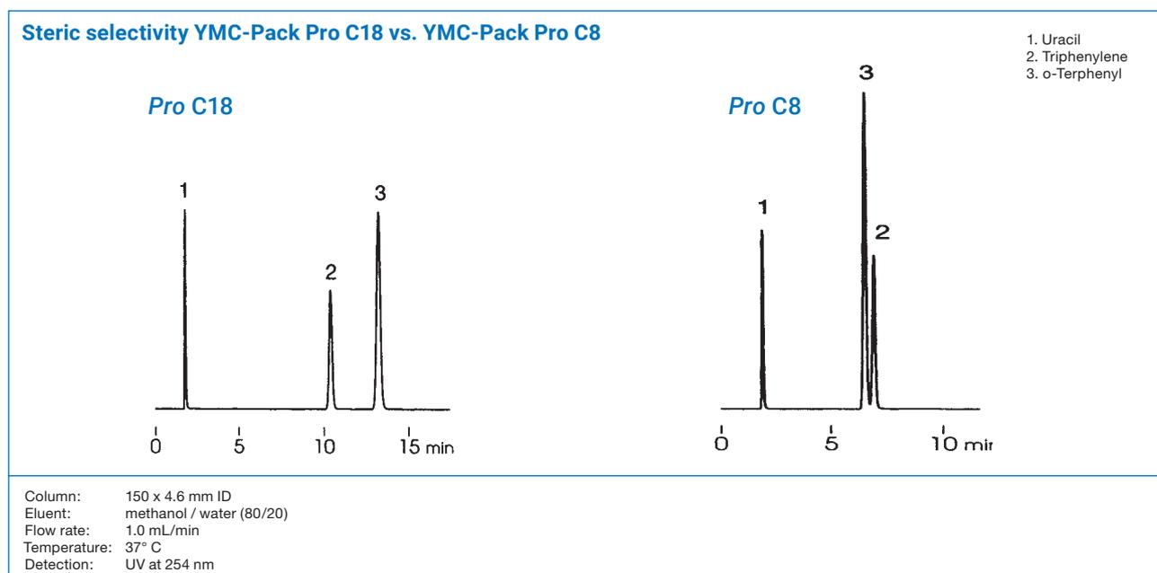
The reversed elution order of triphenylene and o-terphenyl for the shorter C8 chains of YMC-Pack *Pro C8* illustrates the different steric recognition for steric-demanding substances.
