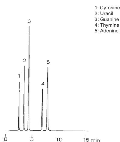
Column: YMC-Pack *Pro C4* (5  $\mu\text{m}$ , 12 nm) 150 x 4.6 mm ID
