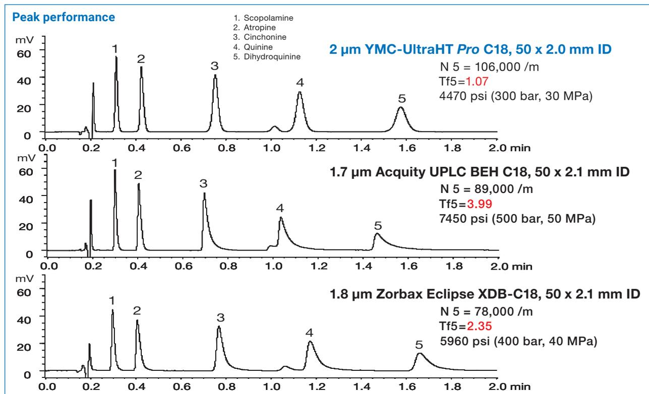
With YMC-UltraHT Pro C18 you have all the efficiency you need to develop your Fast LC methods with none of the pressure or heat some would have you believe is essential!
