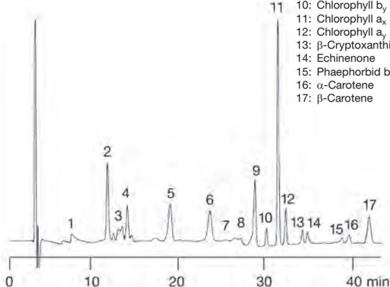
Column: YMC Carotenoid (5  $\mu$ m) 250 x 4.6 mm ID
