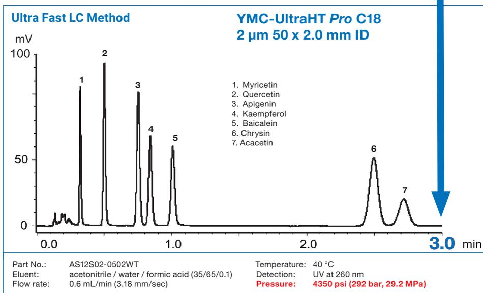
Due to the production processes used to manufacture YMC-Pack Pro-Family, methods can be easily downscaled with unchanged selectivity. As the examples shown demonstrate, conventional HPLC methods can be transferred easily to Ultra Fast LC methods by choosing YMC-UltraHT columns to gain efficiency and significantly reduce analysis time.
