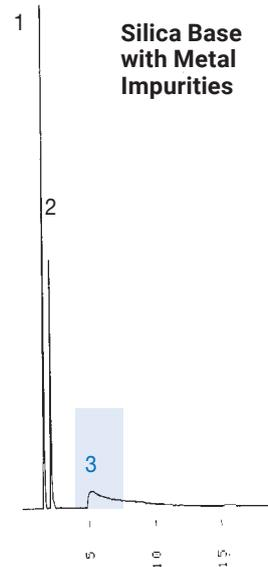
Column: YMC-Pack ODS-A (12 nm, 5  $\mu\text{m}$ ) 150 x 4.6 mm ID
