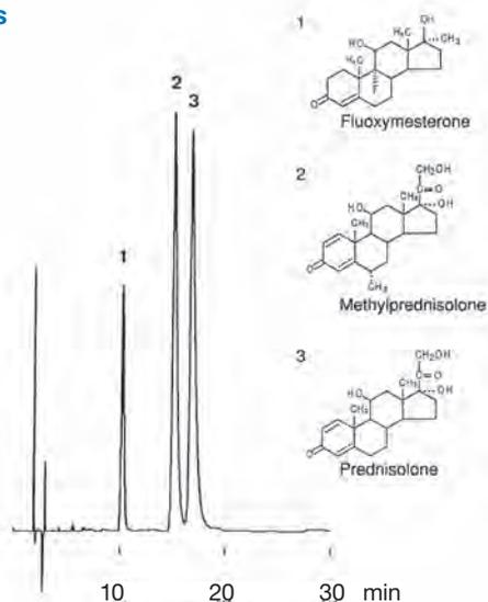
Column: YMC-Pack SIL (5 µm, 6 nm) 250 x 4.6 mm ID
