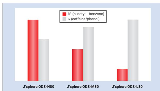
Hydrophobicity (indicated by  $k'$  for n-octyl benzene) and H-bonding capacity (indicated by  $\alpha$  of caffeine/phenol) of J'sphere ODS columns.
