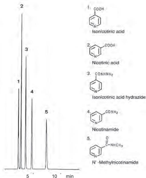
Column: YMC-Pack C<sub>8</sub> (Octyl) (5 μm, 12 nm) 150 x 4.6 mm ID
