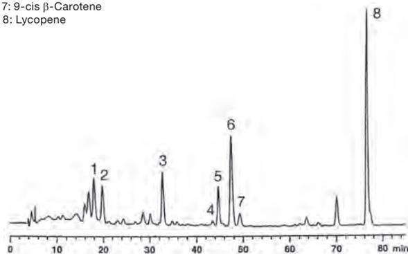
Column: YMC Carotenoid (5  $\mu$ m) 250 x 4.6 mm ID
