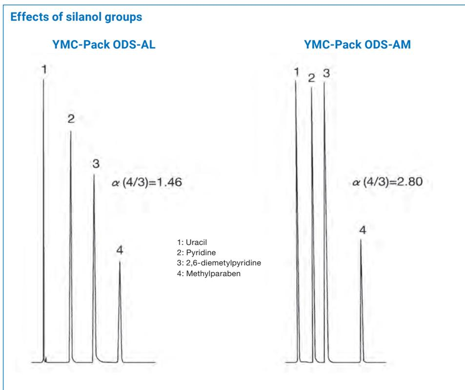
The separation factor ( $\alpha$ ) of internal standards methylparaben / 2,6-dimethylpyridine for YMC-Pack ODS-AL, which is not endcapped is different to that of YMC-Pack ODS-AM. Due to the residual silanol groups, YMC-Pack ODS-AL shows higher retention of pyridines.
