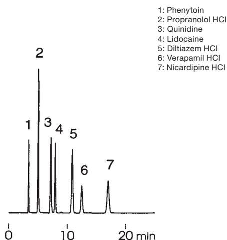
Column: YMC-Pack *Pro C4* (5  $\mu\text{m}$ , 12 nm) 150 x 4.6 mm ID
