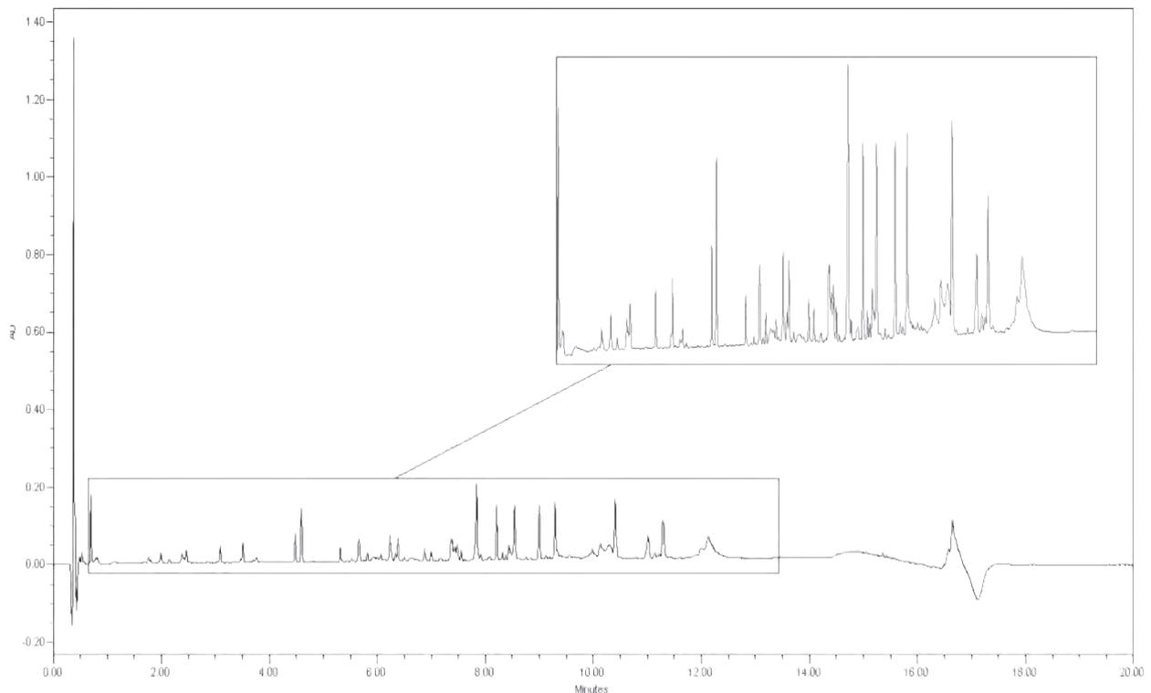
Meteoric Core BIO (2.7 μm, 16 nm) 100 x 2.1 mm ID
