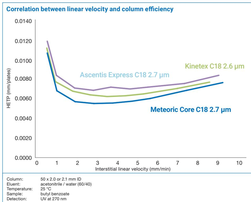
Meteoric Core C18 shows outstanding column efficiencies over a wide flow range.
