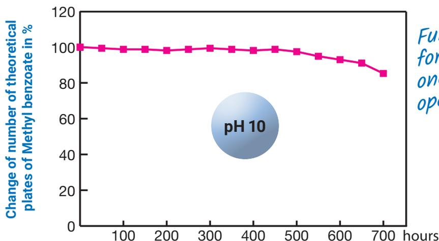
For pH 10, a borate buffer system (20 mM H<sub>3</sub>BO<sub>3</sub>-NaOH (pH 9.8) / methanol 50/50 at 30 °C) was selected to be continuously pumped through the column, while checking the number of theoretical plates for methyl benzoate every 50 hours.
