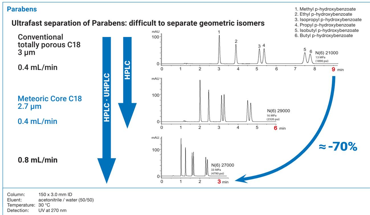
Meteoric Core C18 can shorten the analysis time by two thirds compared to a conventional totally porous C18 column with the same column dimensions and under the same analytical conditions. In addition, it maintains
