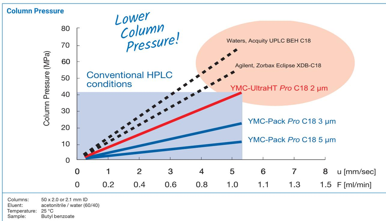
The introduction of YMC-UltraHT Pro C18 2 µm allows easy downscaling of existing methods which use YMC-Pack Pro C18 3 µm and 5 µm.
