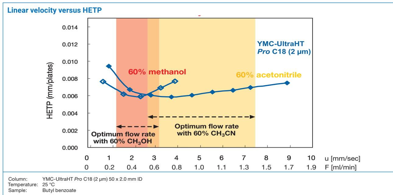
Since YMC-UltraHT columns provide substantially lower pressure drop than most competitive 2 µm or sub-2 µm media, high flow rates can be achieved without generating excessive back pressure and without the need for specialised equipment. Nevertheless, 3 mm ID columns are less
